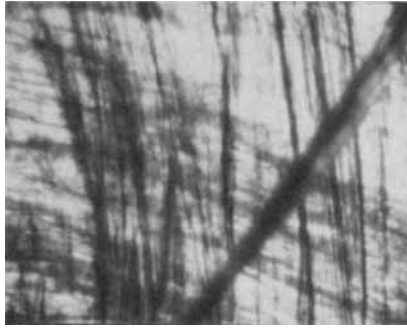
Fig. 6. Type of failure in impact strength tests with multiaxially oriented polyethylene films. The films crack along the residual flow lines in each layer of their laminated structures.
